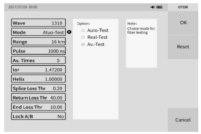
■ Measuring wavelength (nm): Set the test wavelength of OTDR. Setting method: Under the parameter setting interface, the corresponding wavelength can be selected by pressing [Wave], [1310 nm], [1550 nm] or [1310/1550 nm].
