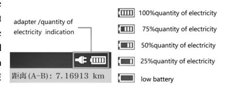
Battery power will be displayed at the top of the screen. When the power is too low, a warning message will appear. Please connect the instrument to the power socket with a random adapter and charge it in time.
