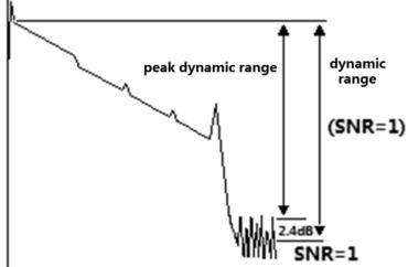
farthest fiber link distance that OTDR can test under the condition of the maximum test pulse width provided by the instrument. Therefore, under the same link condition, the larger the dynamic range, the longer the distance of the optical fiber link that the instrument can test.
