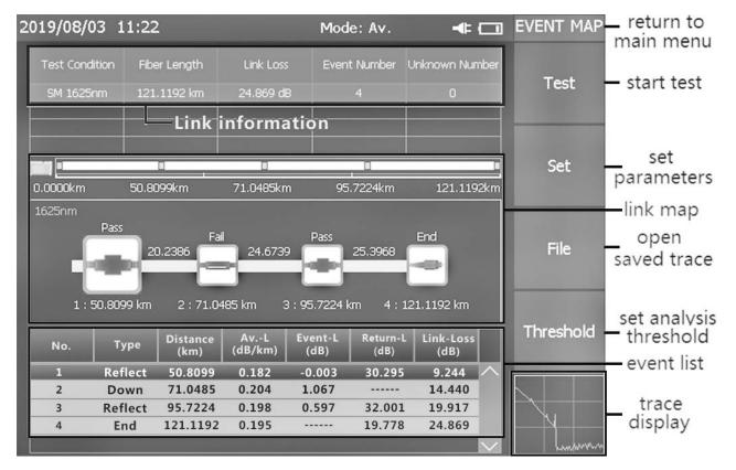
**Splice Loss:** Click on "+" and "-" can increase or decrease the threshold, each step changes 0.02dB, or click the corresponding position of the threshold.
