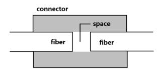
Fresnel reflection at the end of the cable: Fresnel reflection occurs at the breakpoint of the cable or at the position where the group refractive index changes at the end of the cable (glass and air). When the end face of the optical fiber is vertical, the power reflection of the incident light is about 3%(-14.7dB).
