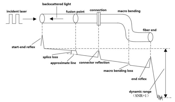
occurring at the junction between OTDR and the connector of the optical cable. This also includes the internal reflection of the instrument, and the loss and reflection between the connecting points cannot be detected in the near-end reflective area.
