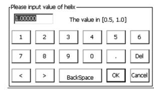
Setting method: Under the parameter setting interface, press [Helix],
