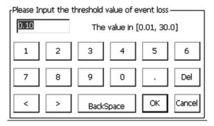
Setting method: Under the parameter setting interface, press [Event Loss Thre.], pop up the event loss
