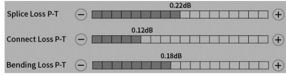
**Connection Loss:** Clicking on "+" and "-" can increase or decrease the threshold, changing 0.25dB per step, or clicking on the corresponding position of the threshold.
