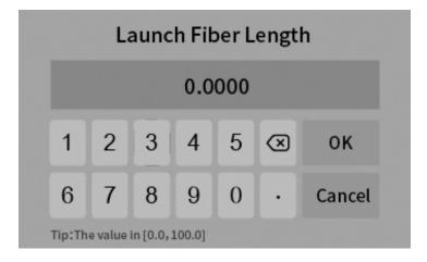
■ Receiving fiber length: used to set the length of OTDR terminal access guide fiber, ranging from 0 to 100. The unit is consistent according to the set unit, which is usually 0 by default.
