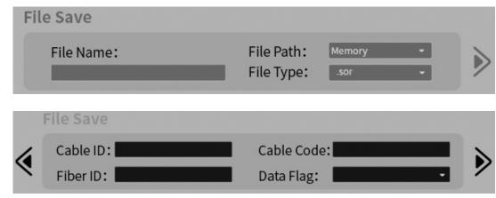
Cable ID and Cable Code set at the initial laying of line.
