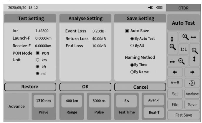
■ Wave: Set the test wavelength of OTDR.
