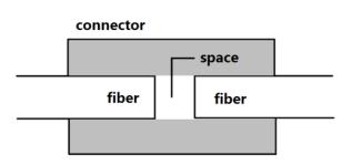
index changes at the end of the cable (glass and air). When the end face of the optical fiber is vertical, the power reflection of the incident light is about 3%(-14.7dB).
