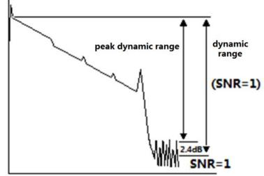
distance that OTDR can test under the condition of the maximum test pulse width provided by the instrument. Therefore, under the same link condition, the larger the dynamic range, the longer the distance of the optical fiber link that the instrument can test.
