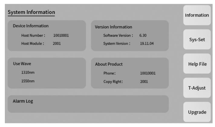
Alarm Log: Record the times the instrument has been tested with light and the latest test with light.
