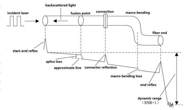
**Near-end reflection:** Reflection occurring at the junction between OTDR and the connector of the optical cable. This also includes the internal reflection of the instrument, and the loss and reflection between the connecting points cannot be detected in the near-end reflective area.
