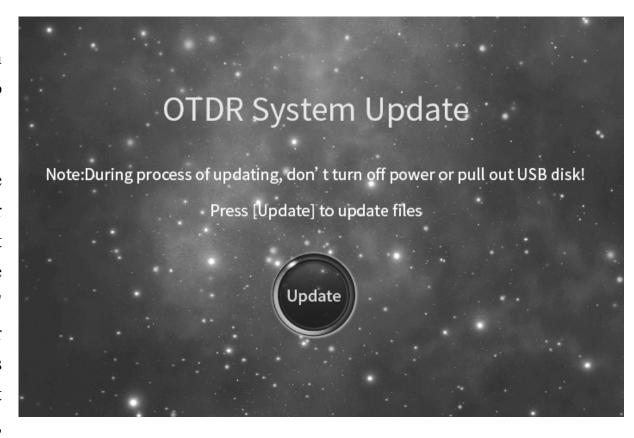
then enter the update interface, click [Update] button, prompt the update completed, restart the instrument. **Note:** When updating, do not turn off or pull out the U disk, otherwise the system will not work properly!
