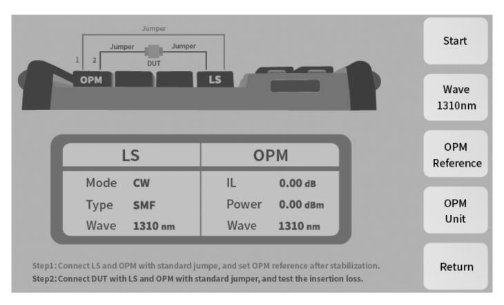
the test piece can be obtained by pressing [Start].
