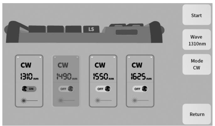
and then press the "ON" below the corresponding wavelength in the wavelength menu or status information to turn off the source of the corresponding wavelength.
